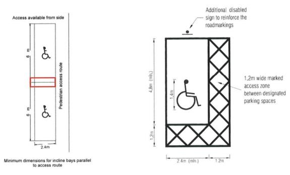
The 1.20m "access zone" can be shared with an adjoining accessible bay. Therefore 12m will be required for the two bays.
