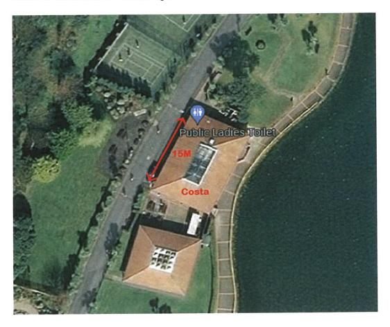
The recommended standard accessible parking bay should be at least 2.40m wide by 3.60m long. In addition, there should be a 1.2m "access zone" around each side of the bay to allow mobility impaired and disabled motorists to get into and out of their vehicles safely i.e. 3.60m wide & 6.00m long. There is insufficient room to provide all the recommended "access zones". The only possible access zones we can install are to the rear of the accessible bays.
