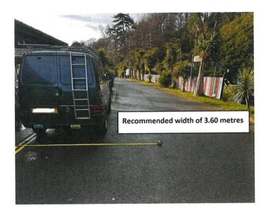
The right-hand side access zone would have afforded protection for the driver and provided sufficient space to open the vehicle door fully when exiting the vehicle, but it is not possible.
